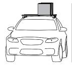
2 Bars 80kg/176lbs 3 bars 120kg/264lbs load rating (Urban road) 2 Bars 53kg/116lbs 3 Bars 80kg/176lbs load rating (Off road - urban / 1.5)
