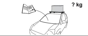
When these roof racks are to be used on a vehicle that is driven off sealed roads, the maximum roof rack load rating should be *divided* by 1.5. Do not forget to subtract 5kg from your maximum carrying capacity due to the weight of the crossbars and legs.
